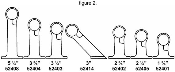
**Standoffs:** Select long standoffs such as 52408 to fit around windshield rails or built-in rod holders. Select standoff 52414 for added reach to fit smaller consoles. Always choose the shortest standoff that will do the job.
